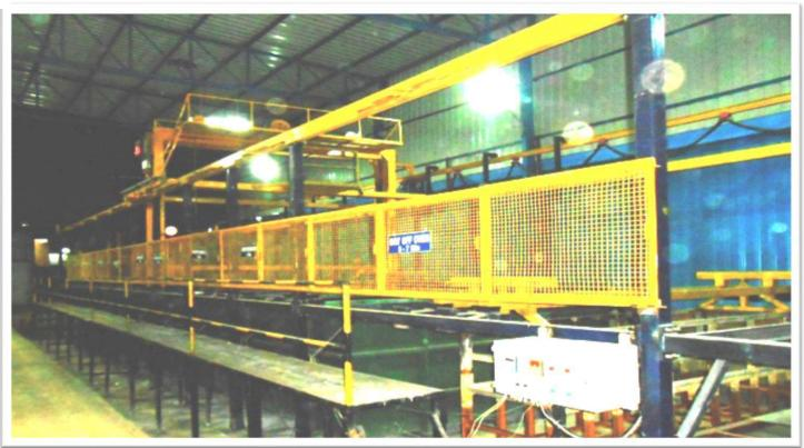
State of art Manual crane transported chromating unit with Semi PLC controlled system by dipping method .
