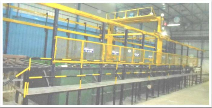
State of art Automated transported phosphating unit with PLC controlled system by dipping method .
